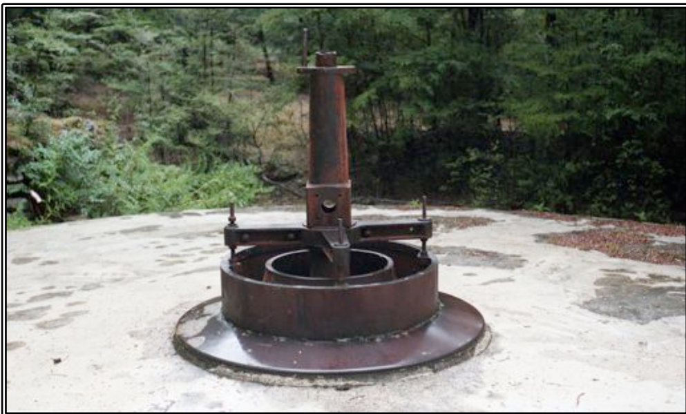
The central pylon on the buddle.
