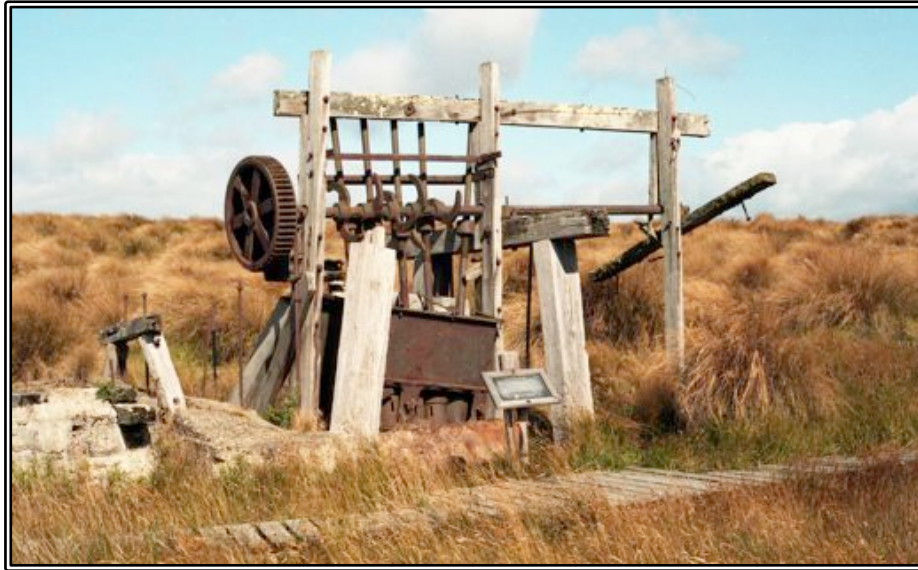
Figure 46 The Canton Battery at Waipori (site H44/831). An example of a trestle-framed stamp mill.
