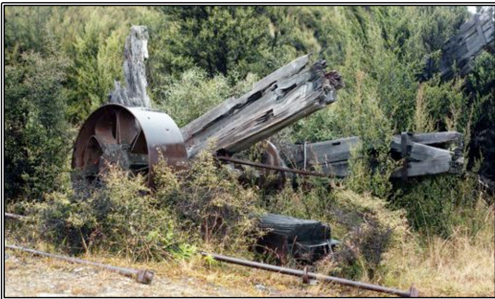
The collapsed stamp mill.
