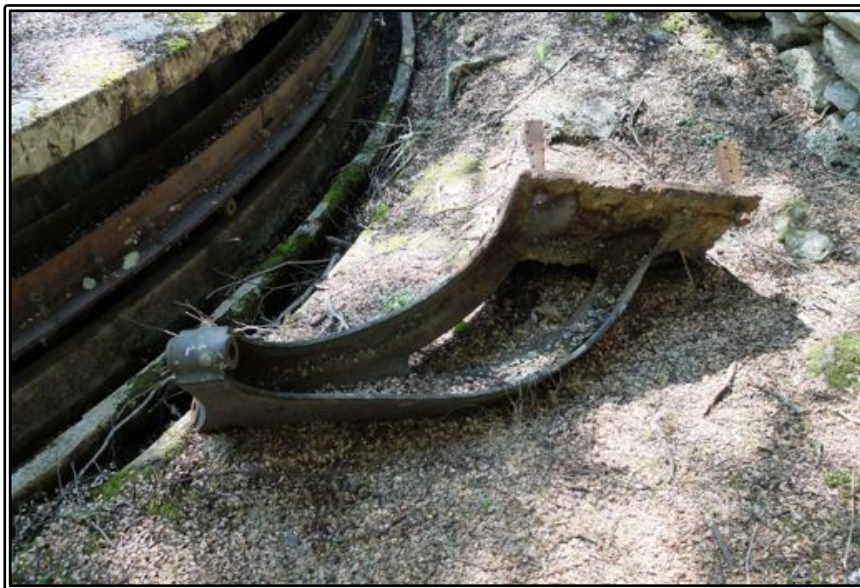
Figure 42 The cast iron arm that used to be mounted beside the buddle, in 2014. It was in place when the site was visited in 1995.
