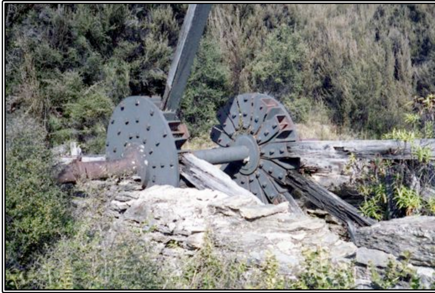
Figure 26 The Invincible water wheel in 1995 (P. Petchey). At this date only a few of the above-horizontal spokes remained in place.
