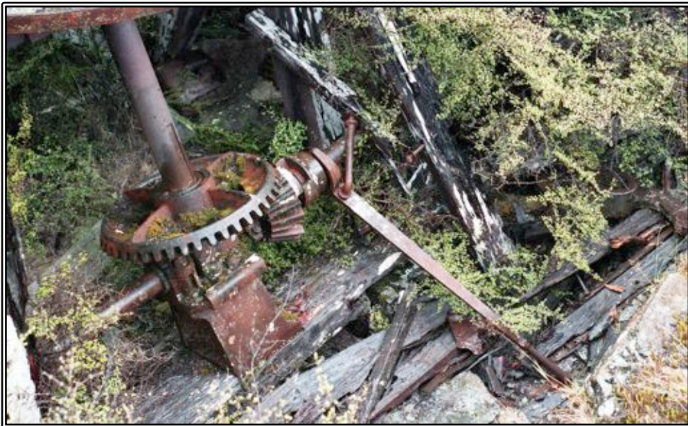
A detail of the drive mechanism of the Berdans.
